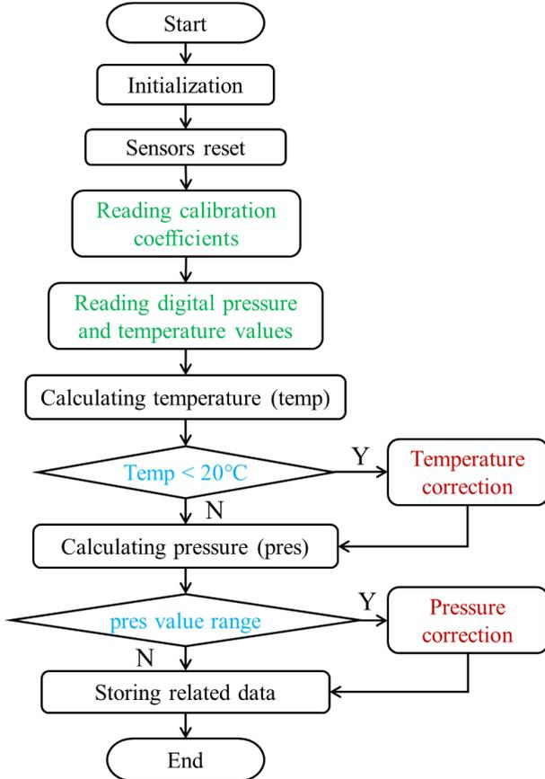
Fig. 7 The process of pressure data acquisition.
