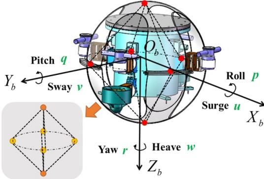
Fig. 3 The SUR-fixed coordinate frame and stereoscopic model of the proposed pressure sensor array.
