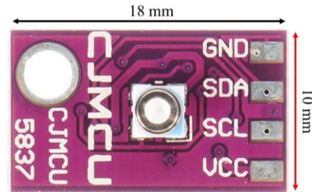
Fig. 2 The pressure sensor of CJMCU-5837.
