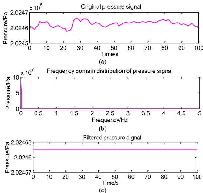
Fig. 10. The signal processing of the sensor #S5 pressure data, including: (a) original pressure signal, (b) frequency domain distribution of pressure signal, (c) filtered pressure signal.
