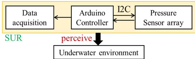
Fig. 6 The proposed detection system for SUR using pressure sensor array.
