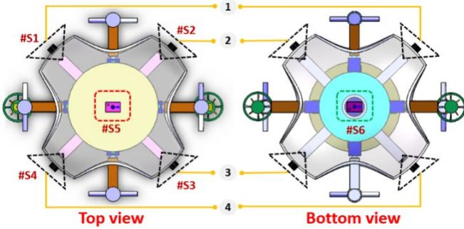
Fig. 4 The proposed sensor array for SUR using pressure sensors.
